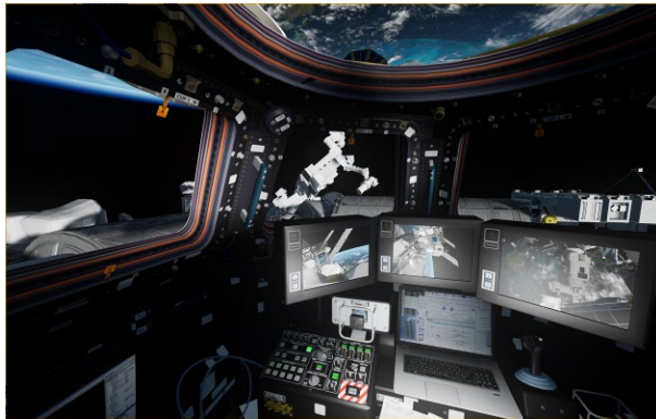
Fig. 15. Life-size representation of the cupola of the ISS in the JIVE-ISS VR application. The robotics monitors are functional and display live views of the station's 3D model.
