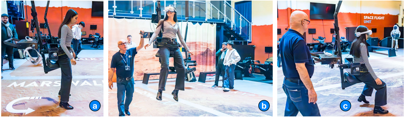
Figure 5: An example of a graviceptive-aware design: a user sitting in a spring chair attached to the ceiling navigating in virtual reality under normal conditions (a), with low-gravity simulation (b), and walking back (c).
