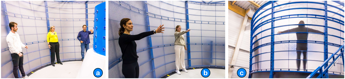
Figure 1: An example of graviception as an embodied mediator in human-computer interaction: end users perform wrist-based horizontal mid-air gestures in a centrifuge with normal gravity (a: 1 g), increased gravity (b: 1.5 g), and maximal gravity simulating a space shuttle at taking off (c: 2.7 g). In the last condition, the end user, almost pressed against the wall of the centrifuge due to the pressure, struggles to perform mid-air gestures.
